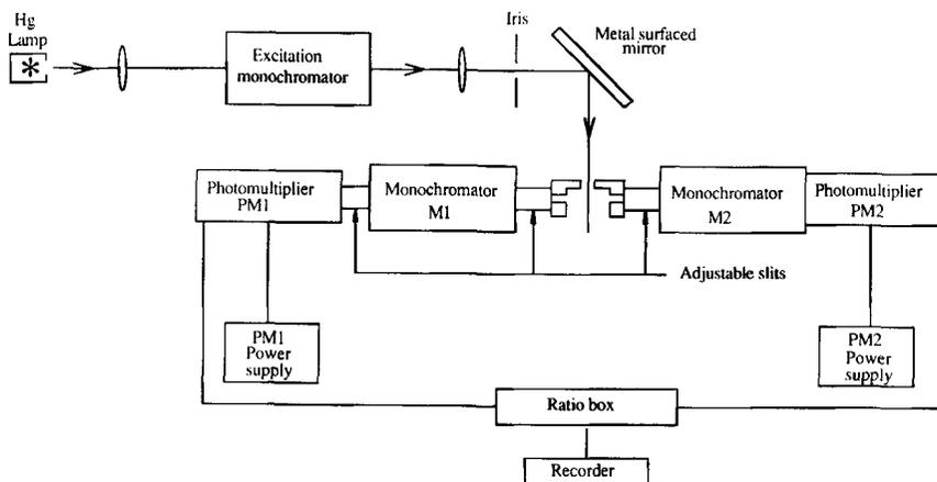
**Figure 2.** Schematic diagram of the chemiluminescence monitoring system showing modification for operation as a simple fluorimeter
