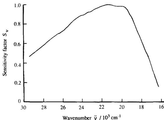
Figure 3. Normalized spectral sensitivity curve
