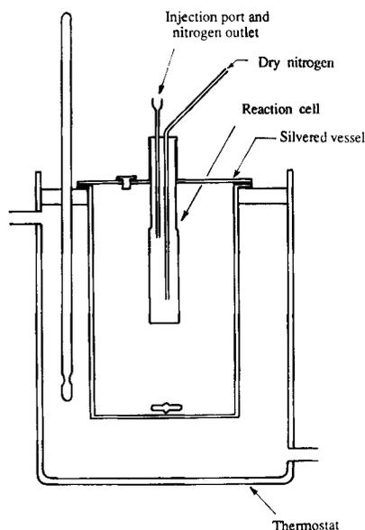
**Figure 1.** Actinometry cell for measurement of absolute chemiluminescence quantum yields
