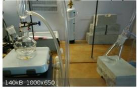
The reaction flask was loaded with 10.6g of NaDCC and 7.5mL of benzene. The addition funnel was attached to the reaction flask and filled with 5mL of deionized water and 7.5mL of ~95% sulfuric acid. Stirring is started and the dilute sulfuric acid is added dropwise. The use of an addition funnel was selected because I expected some immediate chlorine evolution, however none was observed.
