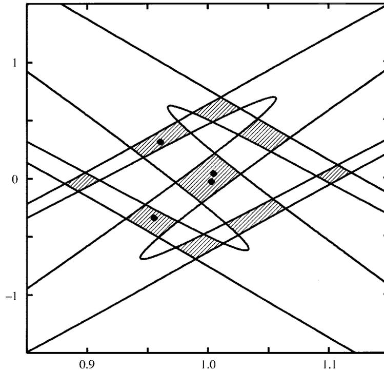
Figure 2. Intersection of forward and backward integration of a range initial conditions which remain around the inverted position  $\theta = \pi$  plotted in  $(\theta, \theta/\pi)$  space. Unstable orbits that oscillate about the unstable inverted position are located in the hatched regions by numerical methods. The position of a period-4 orbit is also shown.
