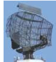
Figure 13: SRE-M7, a typically en-route radar
