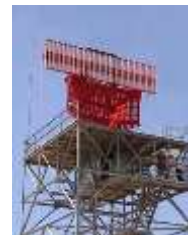
Figure 14: ASR-12, a typically Air Surveillance Radar
