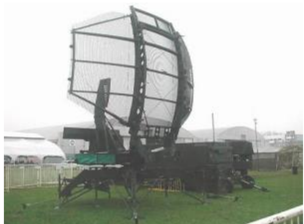
Figure 11: The quite elderly AN/TPS-43 took advantage of pulse compression by phase modulation with the length of 13 codes
