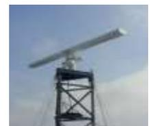
Figure 20: Radar de surface (SMR)
