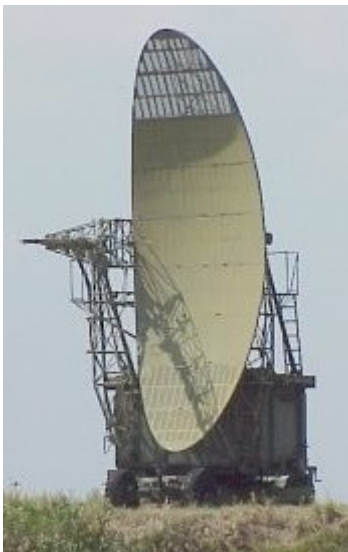
Figure 19: Radar de site PRW-17
