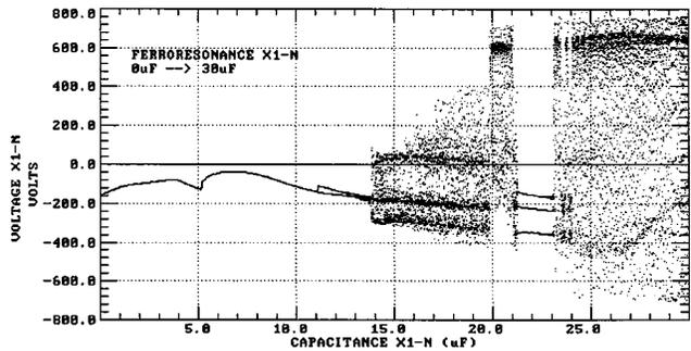
Fig. 13. Sample bifurcation diagram. Shunt capacitance on X1 is ramped from 0 to 30 μF. Blurred areas correspond to chaos.
