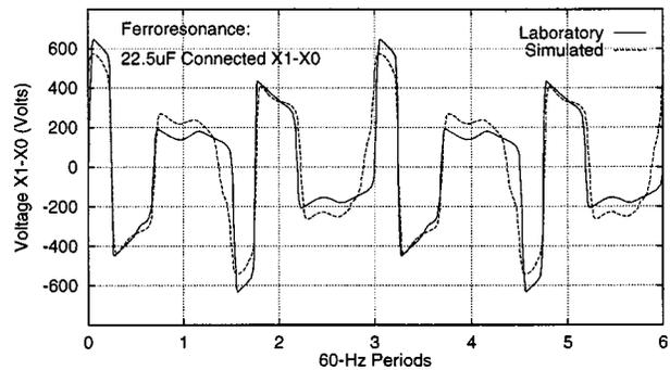
Fig. 14. Period 3 ferroresonance, 22.5 μF connected X1-X0.
