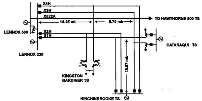
Fig. 16. Ontario Hydro 230-kV system. Ferroresonance involving line X3H and connected transformer at Cataraqui Transformer Station.
