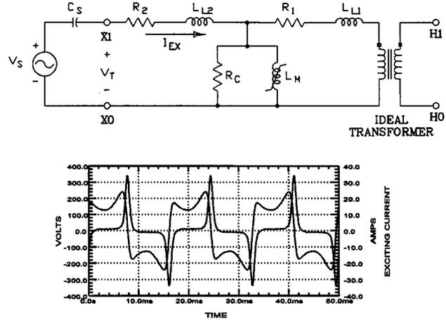
Fig. 2. Same transformer as in Fig. 1, fed through a  $75 \mu\text{F}$  capacitance, operating in ferroresonance. Square waveform is terminal voltage of transformer; spiked waveform is the current.
