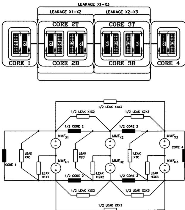
Fig. 8. Development of magnetic circuit for grounded-wye to grounded-wye five-legged wound core transformer. At top, transformer core sectional view used as a basis for duality derivation. Leakage flux paths are labeled. Bold dividing lines mark division in core reluctances. Equivalent magnetic circuit is shown at bottom.
