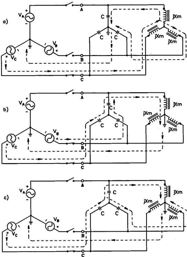
Fig. 4. Three examples of ferroresonance in three phase systems.
