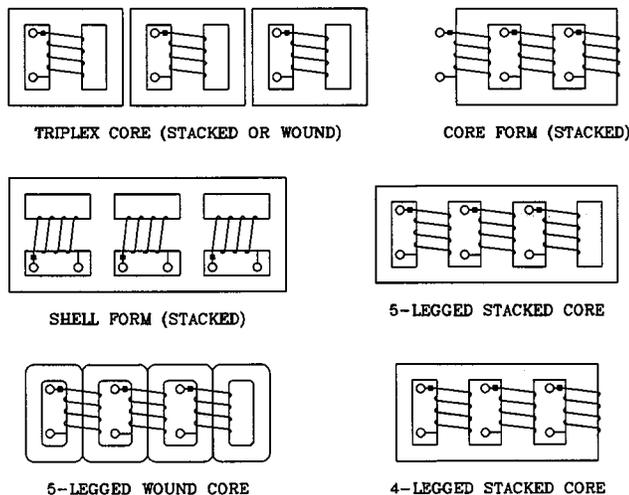
Fig. 3. Core configurations commonly used in three phase transformers. Only one set of windings is shown.
