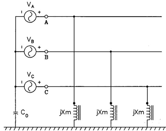
Fig. 12. Reduced system equivalent, neglecting line impedances and lumping all VT's in each phase into an aggregate  $jX_M$ .
