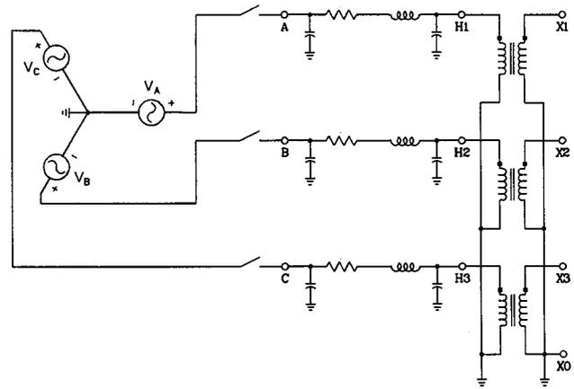
Fig. 5. Typical distribution system supplying a three phase load through a grounded-wye to grounded-wye transformer.
