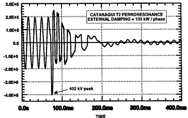
Fig. 18. Cataraqui ( $T2$ ) autotransformer ferroresonance. HV terminal voltage on phase C is 2.0 per unit, with 133 kW/phase of damping.
