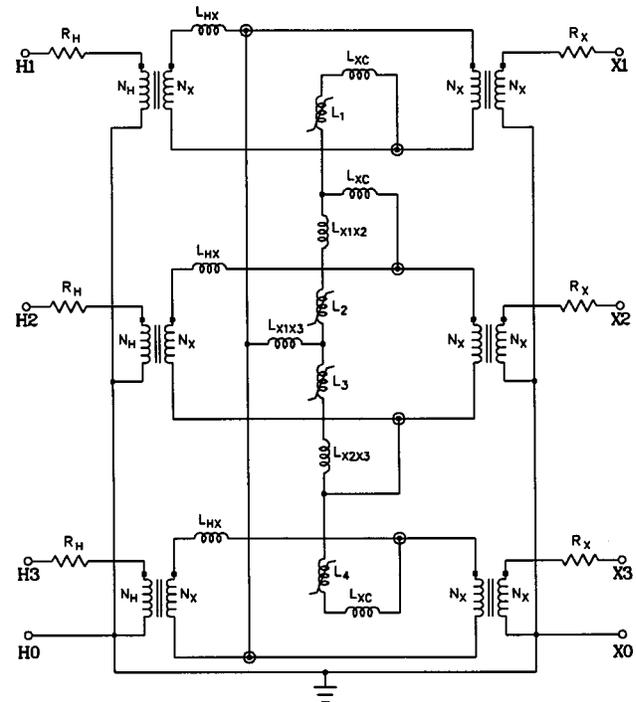
Fig. 9. Duality derived equivalent circuit with current sources replaced by ideal coupling transformers. Winding resistances have also been added.
