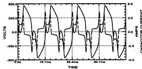
Fig. 6. Measurement of ferroresonance in a three phase grounded-wye to grounded-wye five-legged core transformer. Voltage waveform is solid; current waveform is dashed.
