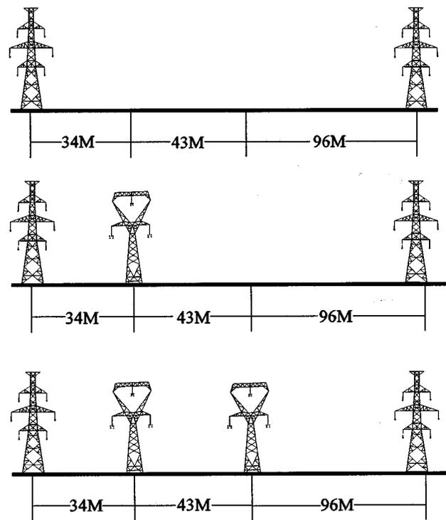
Fig. 17. Sequence of development of the transmission right-of-way.
