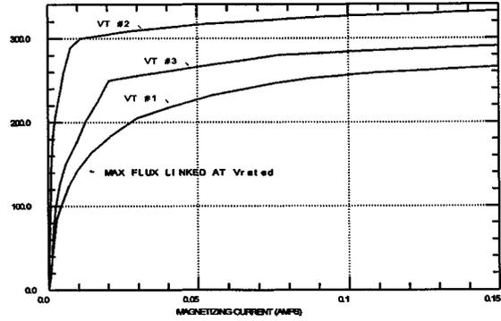
Fig. 11. Comparison of the saturation characteristics of the three VT's. Note the much lower saturation level of VT #1, the ones that were damaged.
