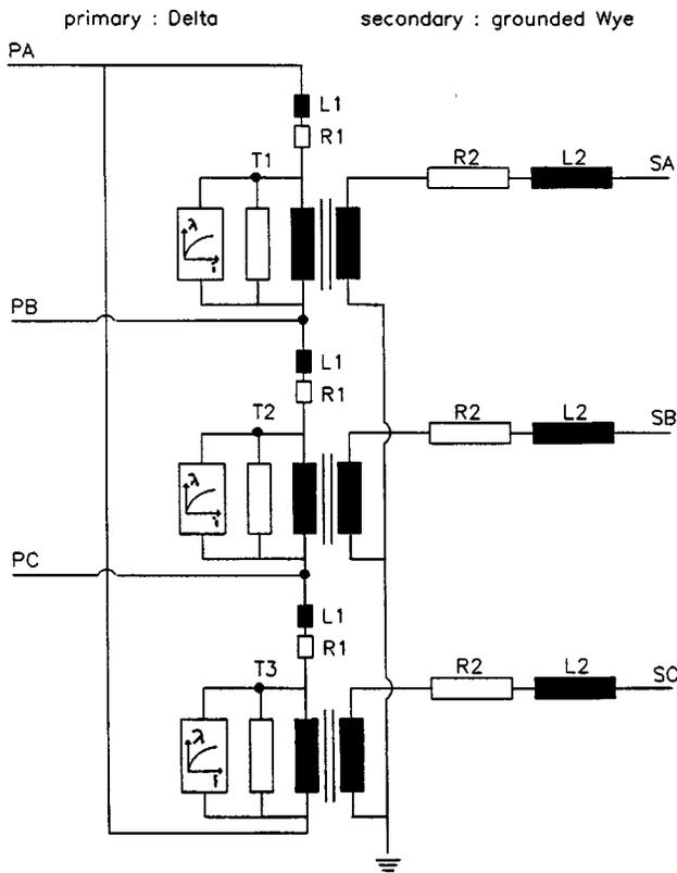
Fig. 7. Model of a delta to wye transformer bank made up of three single phase transformer models [22].
