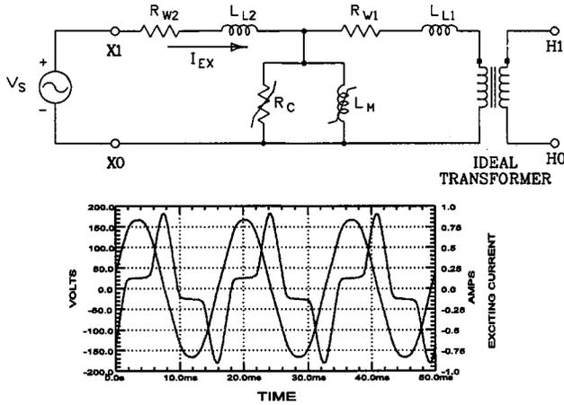
Fig. 1. Unloaded single phase transformer with rated voltage applied. Sine wave is applied voltage; spiked waveform is exciting current.
