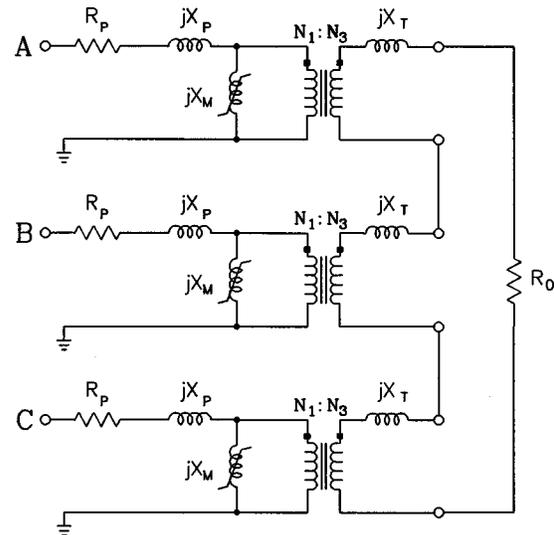
Fig. 10. Typical VT connection in 50-kV Norwegian subtransmission system.
