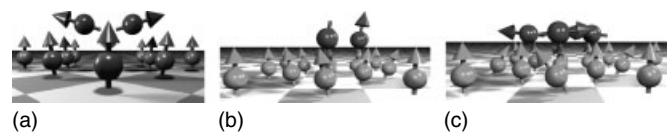
Figure 30. Side view of the magnetic ground-state configuration of a Mn dimer on Ni(100) (Lounis, Mavropoulos, Dederichs and Blügel, 2005) (a), of a Mn trimer (b), and tetramer (c) on fcc Fe(100). In (b), moments of two Mn atoms are pointing down (the second one cannot be seen) and one moment is pointing up.
