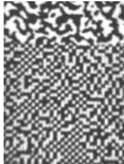
Figure 27. PMOKE image ( 45 \times 35 \mu\text{m}^2 ) of an ac-demagnetized state of the virgin [Pt(0.6 nm)/Co(0.3 nm)] 6 multilayer film (top part of the image), and of the FIB ( D = 10^{14} \text{ Ga ions/cm}^2 ) patterned part (bottom of the image). (P. Warin et al. , Journal of Applied Physics , 90 , 3850 (2001).)
