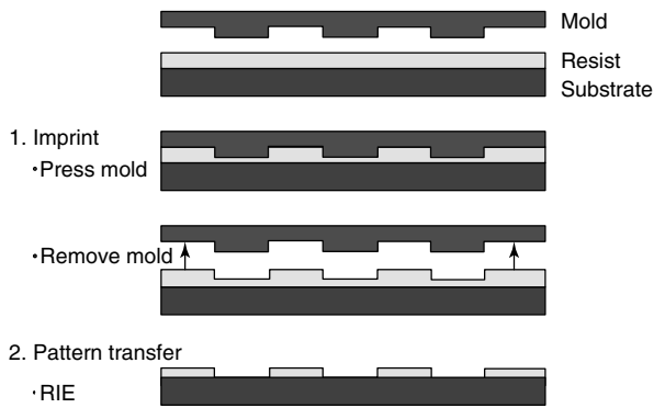
Figure 1. Schematic of nanoimprint lithography process. (1) Imprinting using a mold to create a thickness contrast in a resist; and (2) pattern transfer using anisotropic etching to remove residue resist in the compressed areas (Chou, Krauss and Renstrom, 1995, 1996).
