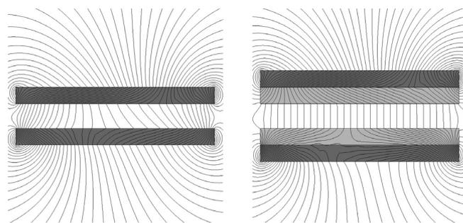
Fig. 5. Iron disks can homogenize a field. Sketches of flux lines with (the right panel) and without (the left panel) iron disks (gray discs) are shown. These are simulations calculated with FEMM [24].
