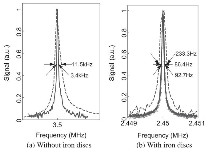
Fig. 6. (a) Hydrogen spectra of doped water with a 5 mm (dashed) and 3 mm (thick) NMR test tube without iron discs and (b) ones with a 5 mm (dashed) and 3 mm (thick) NMR test tube. Nos. 4 and 5 ferrite magnets are selected.  $\Delta$ 's are obtained when Nos. 7 and 8 ferrite magnets are employed. Note that  $\Delta$ 's are shifted from 2.43 MHz for comparison.
