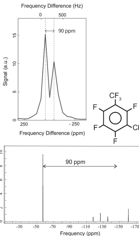
Fig. 9. Spectra of  $^{19}\text{F}$  in 3 chloro-2,3,4,5,6 tetrafluoro-benzo-trifluoride. The upper left panel shows a spectrum measured with our magnet, while the lower panel with a commercial NMR spectrometer (ECA-500, JEOL Resonance) at 11.75 T. The upper right panel is a structure of this molecule.
