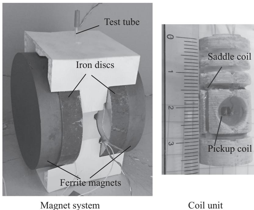
Fig. 4. The white magnet base is monolithic and printed by a 3D printer. The magnet system is placed in a styrene foam box in order to stabilize its temperature. It does not require extra electric shields. The coil unit contains the pickup and saddle coils and is placed in the center of the magnet system, as shown in Fig. 1. The coil bobbin is also printed.
