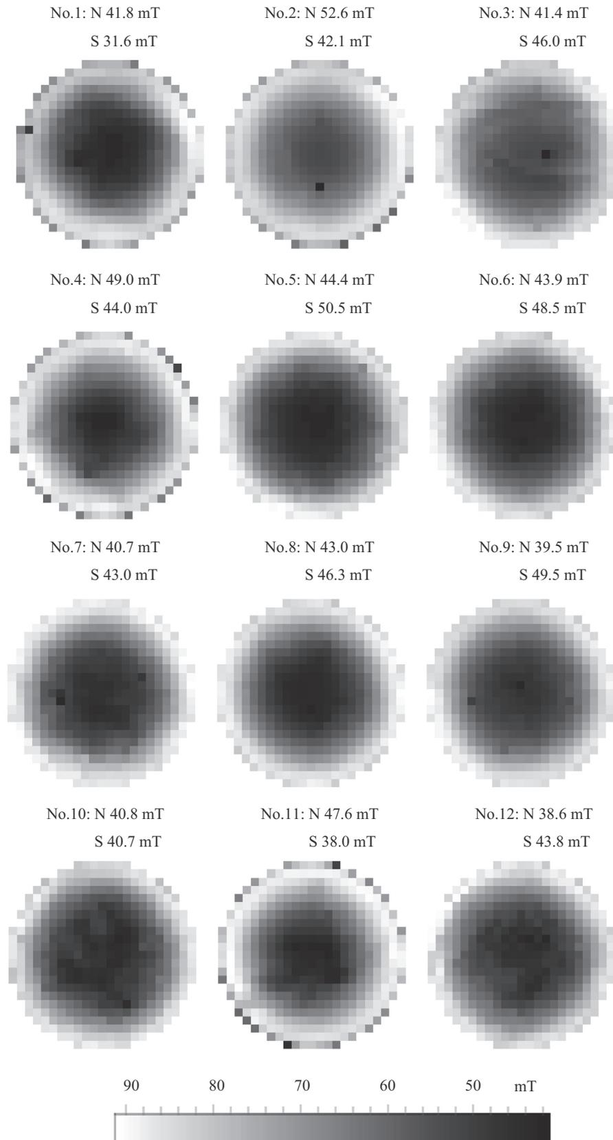
**Fig. 2.** Measured fields at 1.6 mm above the surfaces of the north sides of twelve ferrite magnets. The intervals between measured points are 5 mm. The magnetic fields at the center of both the north and south sides are shown, as well. The fields of the south sides are measured only at the centers.
