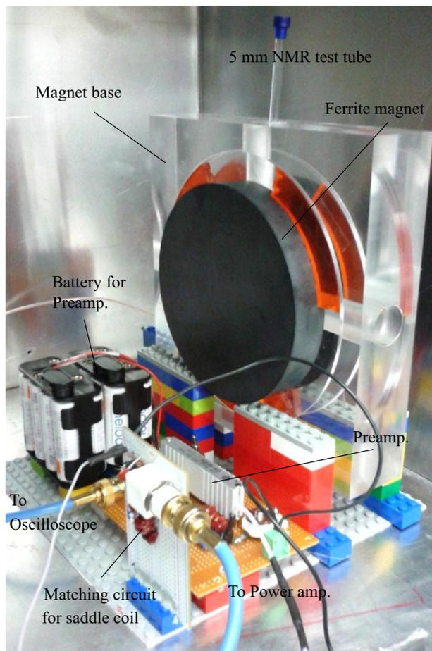
Fig. 3. The magnet system made of acrylic and electronics for measurements.
