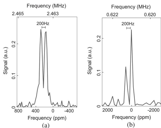
Fig. 8. Spectra of chloroform. (a)  $^1\text{H}$  and (b)  $^{13}\text{C}$  spectra are measured with our NMR magnet system. The scalar coupling constant between  $^1\text{H}$  and  $^{13}\text{C}$  is measured to be 215 Hz with a commercial NMR spectrometer (ECA500, JEOL Resonance) at 11.75 T.
