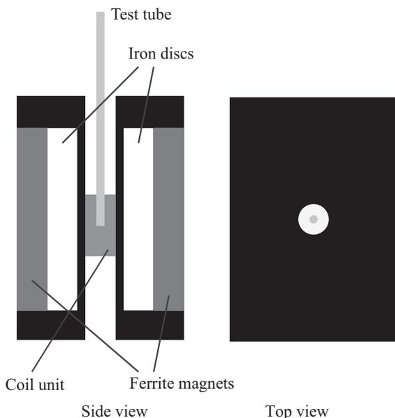
**Fig. 1.** Sketch of our NMR magnet system. The black part is a magnet base on which the ferrite magnets and iron discs are set with their magnetic attractive forces. The coil unit contains the pickup and saddle coil.
