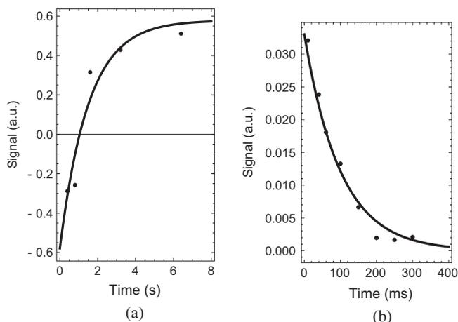
Fig. 7. Typical (a)  $T_1$  and (b)  $T_2$  measurements of the water sample.
