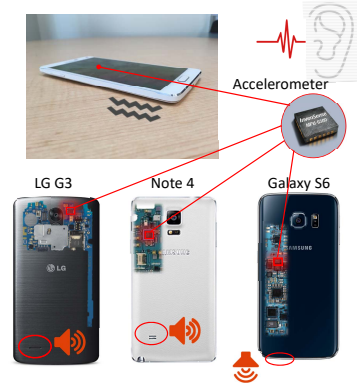
Fig. 6: The speaker and the sensor positions on the smartphones of different vendors.
