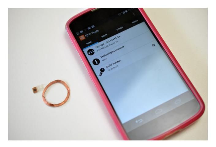
If using a larger tag, you will need to rewind the antenna coil to fit your finger. Be careful not to scratch or break the thin enameled antenna wire!
