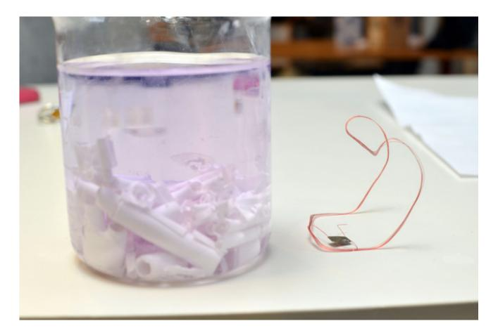
You can also take a bigger tag like the business card-size one pictured above, and dissolve away the plastic with acetone (cover with plastic and a rubber band and keep in a well-ventilated space until the antenna and chip can be easily removed).
