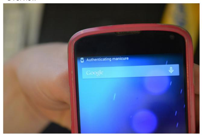
Unlock your phone by just picking it up! No more pesky password or gesture PIN, just scan an NFC tag! This guide covers creating an NFC ring, putting an NFC tag in your nail polish, modding your Android installation to read tags from the lockscreen, and creating an automation toolchain to unlock the phone when the desired tag is scanned.
