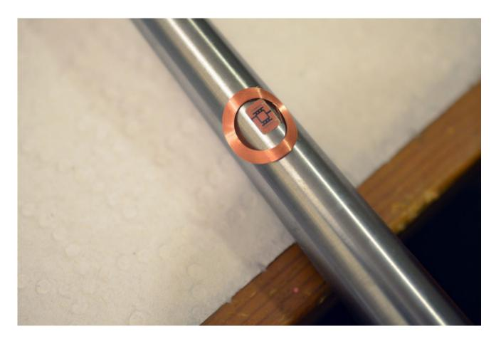
Curve the antenna coil over a round object like a ring mandrel. The tag should fit snugly to the curve of your nail without springing up away from it.
