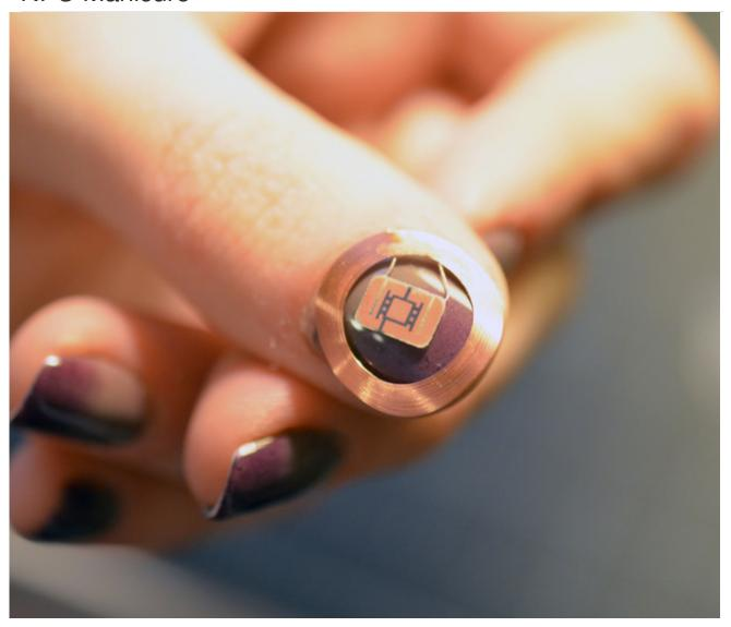
Another way to put NFC tags on your hand is to laminate one into your nail polish! We pulled this small tag out of one of the leather fobs in the store, and trimmed the plastic close to the antenna until the layers peeled apart, then removed any stick residue with rubbing alcohol.
