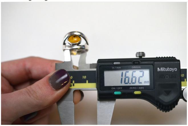
Measure your finger or ring that fits well to determine what size to go for-- then seek out RFID tags with a coil close to this same diameter.
