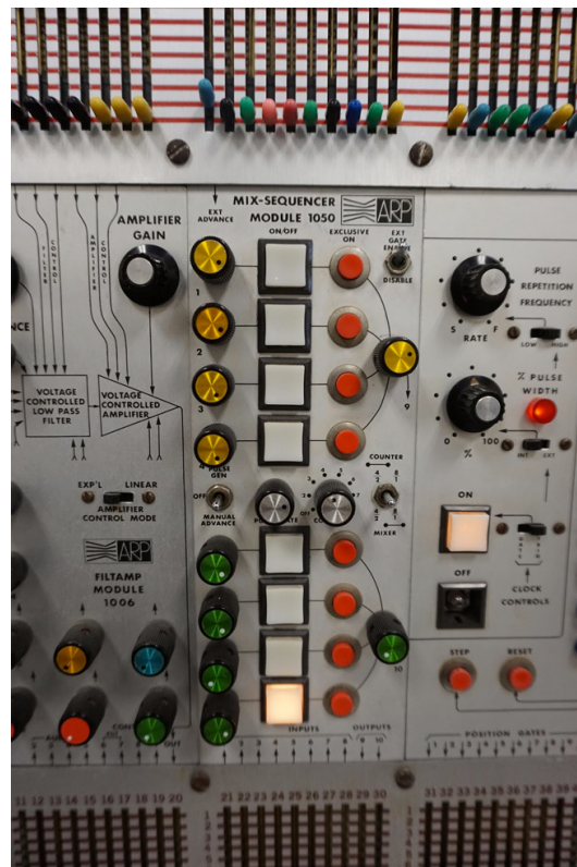
1050 Mix-Sequencer Module in the center with 1006 Filamp module to the left
