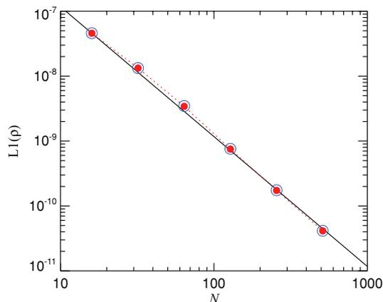
**Figure 19.** L1 error norm for an acoustic wave in 1D, calculated with the moving-mesh code (red circles), or with a fixed mesh (blue open circles). The two schemes produce nearly identical errors (the moving-mesh code lies only  $\sim 1$ – $2$  per cent lower), and the solution converges as  $L1 \propto N^{-2}$ , i.e. with second-order accuracy.
