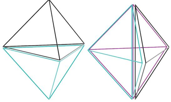
**Figure 4.** The standard replacement operation in 3D required for restoring Delaunayhood. It consists of 2-to-3 (from left to right) or 3-to-2 (from right to left) flips of tetrahedra. Note that the 2-to-3 flip is only possible if the line connecting the two points opposite of the common face intersects the interior of this face. Conversely, the 3-to-2 flip is only possible if an edge is shared by exactly three tetrahedra.
