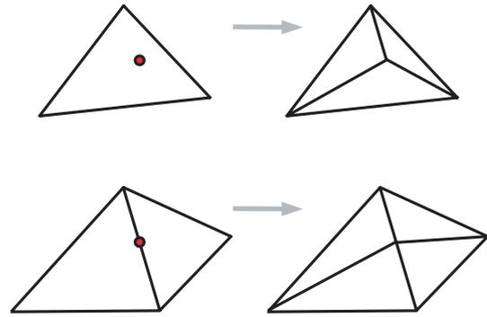
**Figure 5.** Point insertion in 2D in the normal case (top, via a 1-to-3 flip) and the degenerate case (bottom), where the point lies *exactly* on an edge of the current tessellation. In the latter case, the two triangles need to be replaced with four triangles (a 2-to-4 flip).
