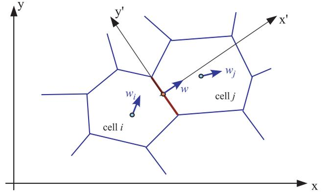
**Figure 10.** Geometry of the flux calculation. We use an unsplit scheme where the flux across each face is estimated based on a 1D Riemann problem. To this end, the fluid state is expressed in a frame which moves with the normal velocity  $\mathbf{w}$  of the face, and is aligned with it. Note that the motion of the face is fully specified by the velocities of the mesh-generating points of the cells left and right of the face.
