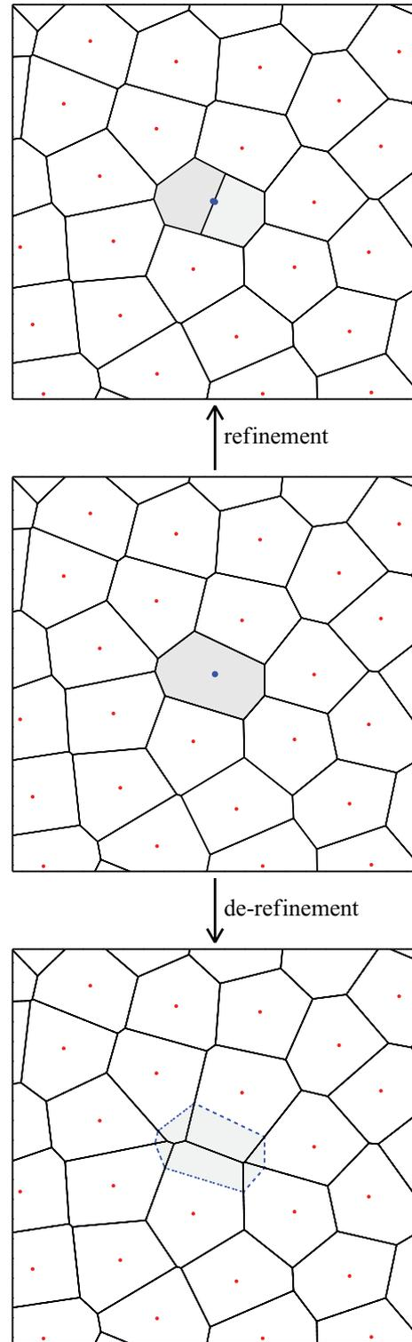
**Figure 16.** Example for the mesh refinement and de-refinement operations. In the middle panel, a Voronoi cell is marked in grey. In a refinement operation, the cell is split into two cells, as shown in the top panel. If a coarsening of the mesh resolution is desired, the cell may be eliminated from the mesh in the derefining operation shown in the bottom panel.
