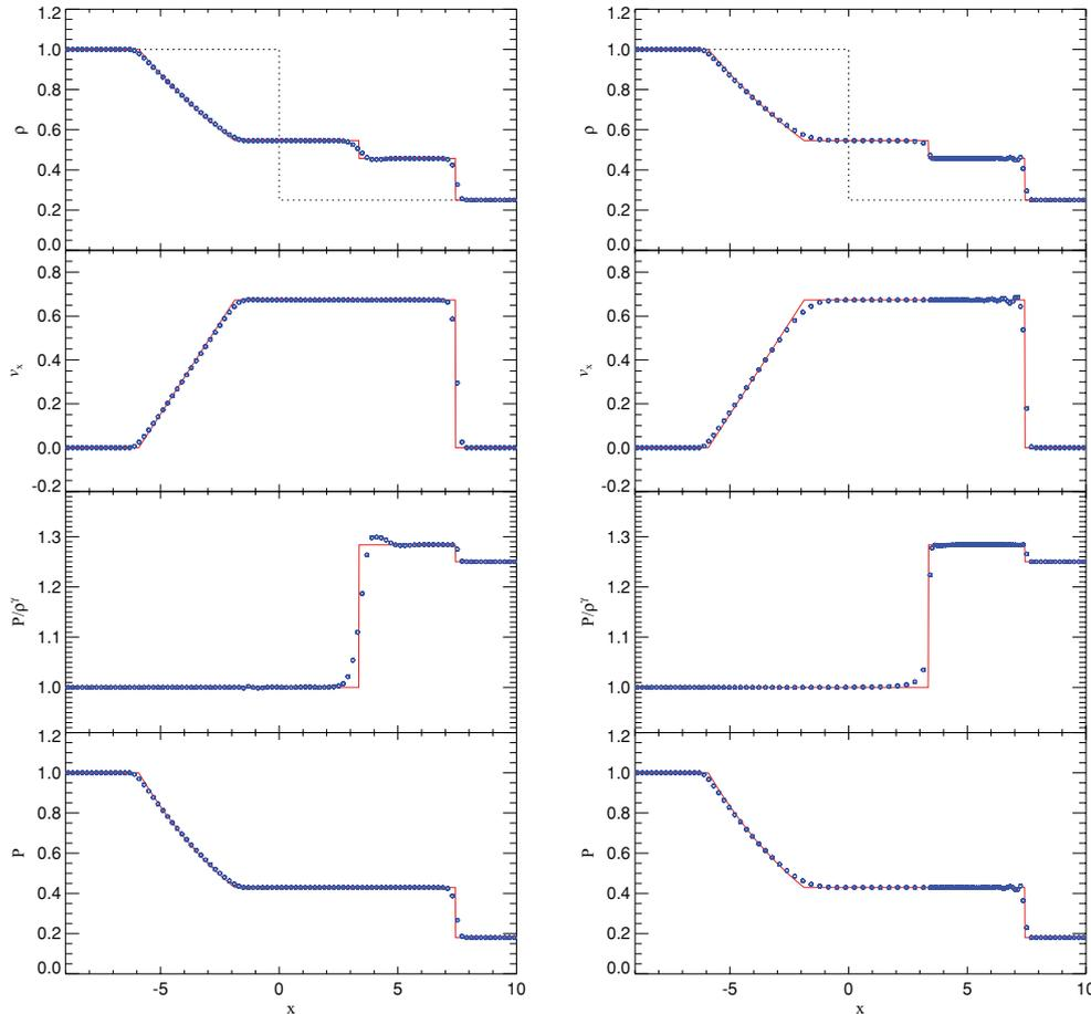
**Figure 21.** A shock tube test with initial conditions frequently used in previous code tests (Hernquist & Katz 1989; Rasio & Shapiro 1991; Wadsley et al. 2004; Springel 2005). The panel on the left shows the result (symbols) of a 2D test with equal volume per cell and a fixed mesh, the right when the mesh is allowed to move. The solid lines show the analytic solution, and the dotted lines in the top row mark the initial conditions.
