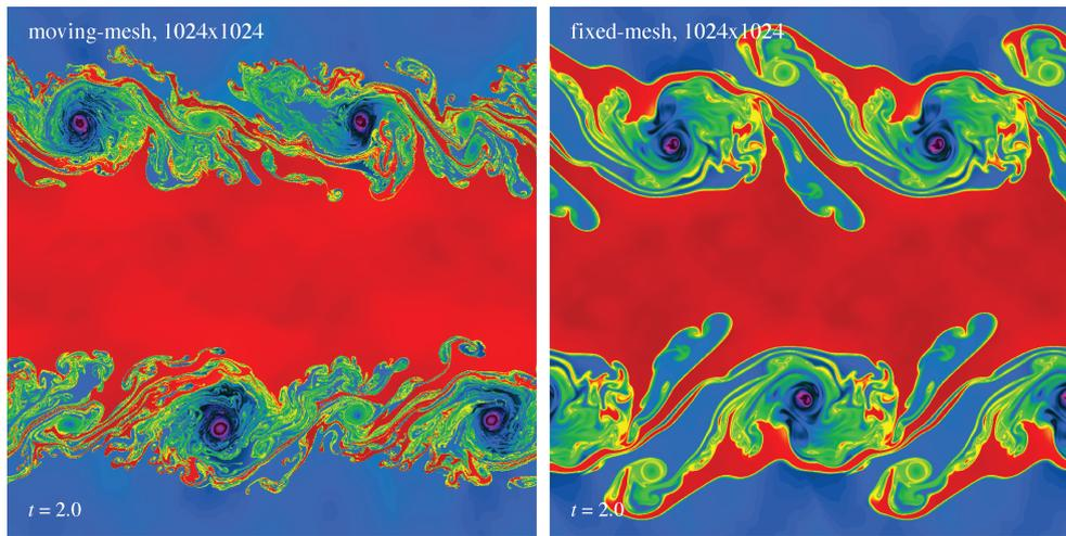
**Figure 34.** KH instability test at high resolution, using a  $1024 \times 1024$  initial mesh. We compare results obtained with the moving-mesh approach (left-hand panel) to those on a fixed grid (right panel), at time  $t = 2.0$ . Quite strikingly, small-scale features of the flow are preserved in the moving-mesh code with much less mixing, albeit at the price of earlier generation of asymmetries in the flow.
