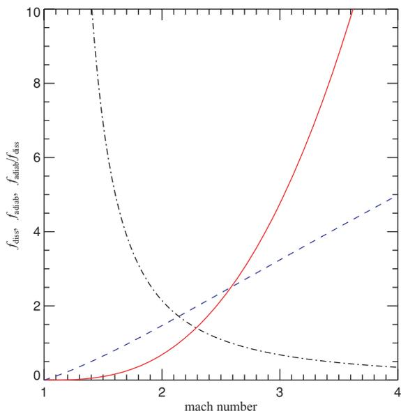
**Figure 12.** Dissipative heating rate  $f_{\text{diss}}(\mathcal{M})$  in a shock as a function of Mach number  $\mathcal{M}$  (red solid line), for a  $\gamma = 5/3$  gas. The dashed blue line gives the adiabatic heating rate  $f_{\text{adiab}}(\mathcal{M})$  of the gas as it is compressed at the shock. Finally, the dash-dotted line gives the ratio of adiabatic and dissipative heating rates.
