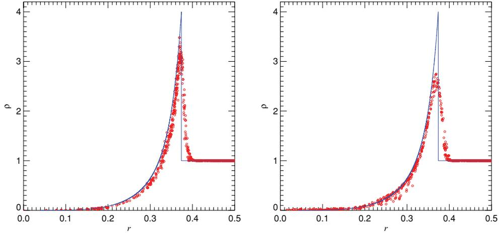
**Figure 25.** Density profile for a 3D Taylor–Sedov blast wave calculation at time  $t = 0.06$ . The initial resolution was  $64^3$  cells, with all the explosion energy injected into a single cell. We compare results for our moving-mesh code (left-hand panel) with the result obtained for a fixed Cartesian mesh (right-hand panel). The circles give the densities of individual cells, which have been randomly subsampled by about  $1/200$  to avoid too strong crowding.
