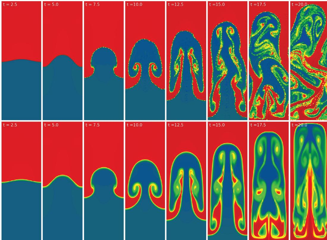
**Figure 35.** Time evolution of a RT instability in simulations with a moving (top) and a static (bottom) mesh. The resolution is quite low, only  $48 \times 144$  cells have been used for this test.
