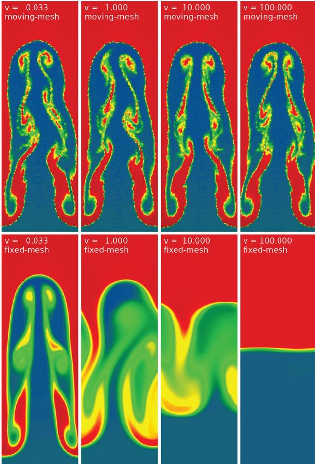
**Figure 36.** RT instability calculated with different Galilean boosts  $v_x$  in the horizontal direction (the simulation domain is periodic in the  $x$ -direction). The correct result should in principal be independent of  $v$ . The top row shows the result at time  $t = 15.0$  computed with our moving-mesh approach, while the bottom row of panels gives the corresponding results for a fixed-mesh calculation with AREPO.
