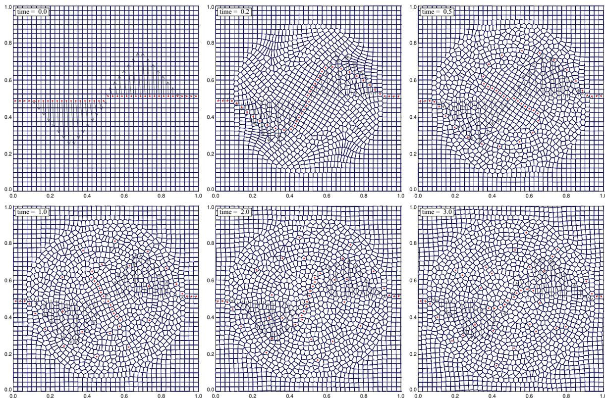
**Figure 27.** Mesh-motion in the ‘triangular’ vortex problem of Gresho, calculated with a  $40 \times 40$  grid of particles. One horizontal row of particles in the initial distribution is marked with circles, and the same cells are labelled with circles in all subsequent frames.
