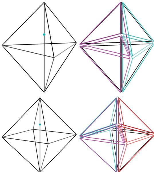
**Figure 7.** Degeneracy during point insertion in 3D. Here, the point that is to be inserted falls on to an edge of the current tessellation. In this case, we need to make an  $n$ -to- $2n$  flip, where  $n$  is the number of tetrahedra that have the edge in common. In most cases this is either three (top left) or four (bottom left), like in the examples shown in this figure, but  $n$  can in principle also be larger.
