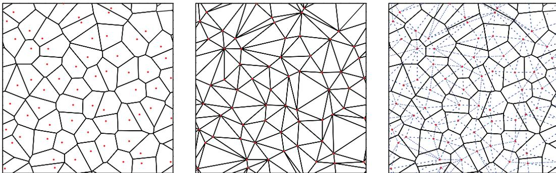
**Figure 1.** Example of a Voronoi and Delaunay tessellation in 2D, with periodic boundary conditions. The panel on the left-hand side shows the Voronoi tessellation for  $N = 64$  points (shown as red circles); the panel in the middle gives the corresponding Delaunay tessellation, while the panel on the right-hand side shows both simultaneously (the solid lines show the Voronoi and the dashed lines the Delaunay tessellation).
