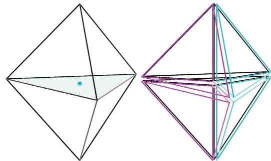
**Figure 6.** Degeneracy during point insertion in 3D. Here, the point that is to be inserted falls on to a face of the current tessellation. The two tetrahedra involved need to be replaced by six tetrahedra, constituting a 2-to-6 flip.
