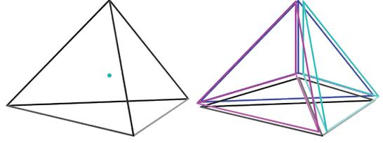
**Figure 3.** A '1-to-4' flip. A newly inserted point splits its insertion tetrahedron into four daughter tetrahedra.
