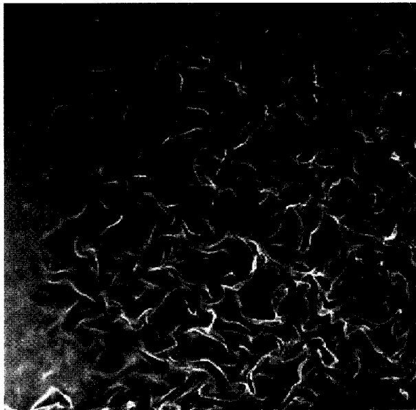
Fig. 1.13. Wrinkling of a fluid surface in isotropic turbulence (Van Dyke 1982). Photograph M. Karweit.
