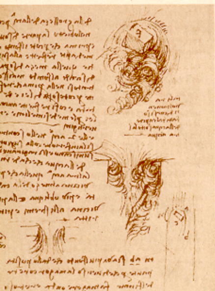
The figure on the upper right part of the cover shows a turbulent flow past an object (from Leonardo da Vinci, ms. F, p. 18v, Bibliothèque de l'Institut de France).
