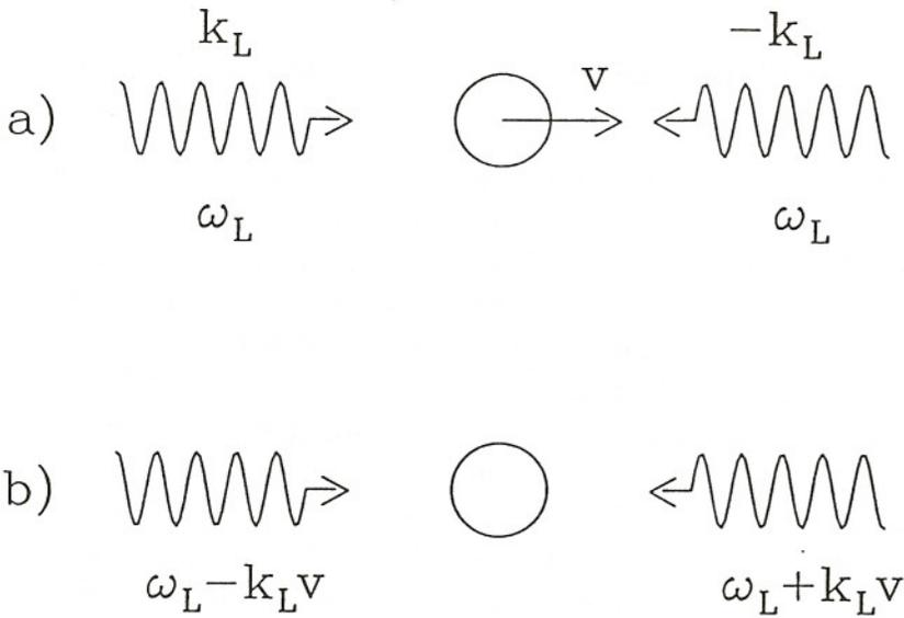
Figure 1: The laser waves of the Doppler cooling configuration, in the lab (a) and in the atomic rest frame (b).
