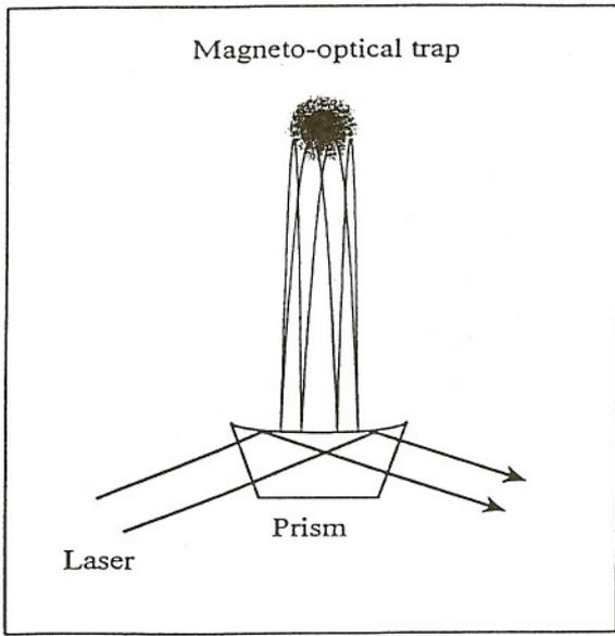
Figure 10: *Principle and loading of the atomic gravitational cavity.*
