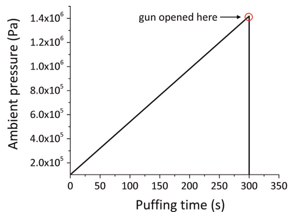
Fig. 31. Ambient pressure at the boundary of the rice kernel for the gun-puffing process.
