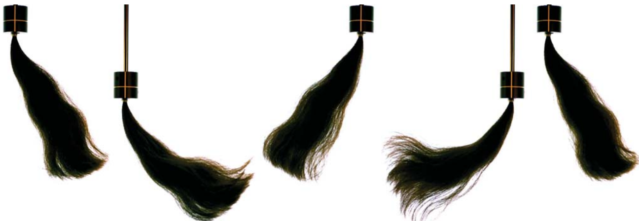
FIGURE 4. A SWINGING PONYTAIL. When a ponytail's support is oscillated vertically at 2.5 Hz, a subharmonic parametric instability is triggered, in which the ponytail swings from side to side. Viewed left to right, the ponytail executes one complete cycle of sideways motion in the time taken by the support to move vertically through two cycles. (Images by James Moore, Philip de Friend, and Ray Goldstein.)
