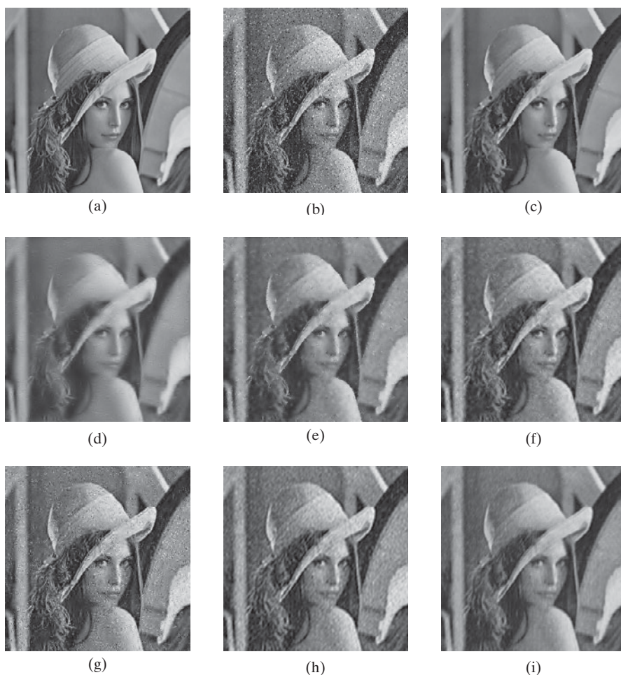
FIGURE 8.15 Denoising an image corrupted by salt and pepper noise. (a) Original image of Lena. (b) Input noisy image. (c) Median filter. (d) Matlab's wavelet denoising. (e) Matlab's Wiener filter. (f) Choi and Baraniuk's method. (g) Pižurica and Philips's method. (h) PCA ( r = 20 ). (i) KHA ( r = 20 ). (This figure is reproduced with the permission of Dr. K. I. Kim.)
