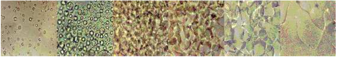
Figure 1.21: Cosmological-defect formation can be simulated in the laboratory by observing the transformation of liquid crystal between phases with different optical properties. In this sequence, bubbles of a new phase nucleate in an initially uniform liquid. As the bubbles grow and coalesce, their boundaries develop into structures analogous to cosmic strings. The scale of the pattern grows similarly to the way the scale of a network of cosmic strings increases with cosmic expansion. (Images courtesy of Ajit Srivastava, Institute of Physics, Bhubaneswar, India.)
