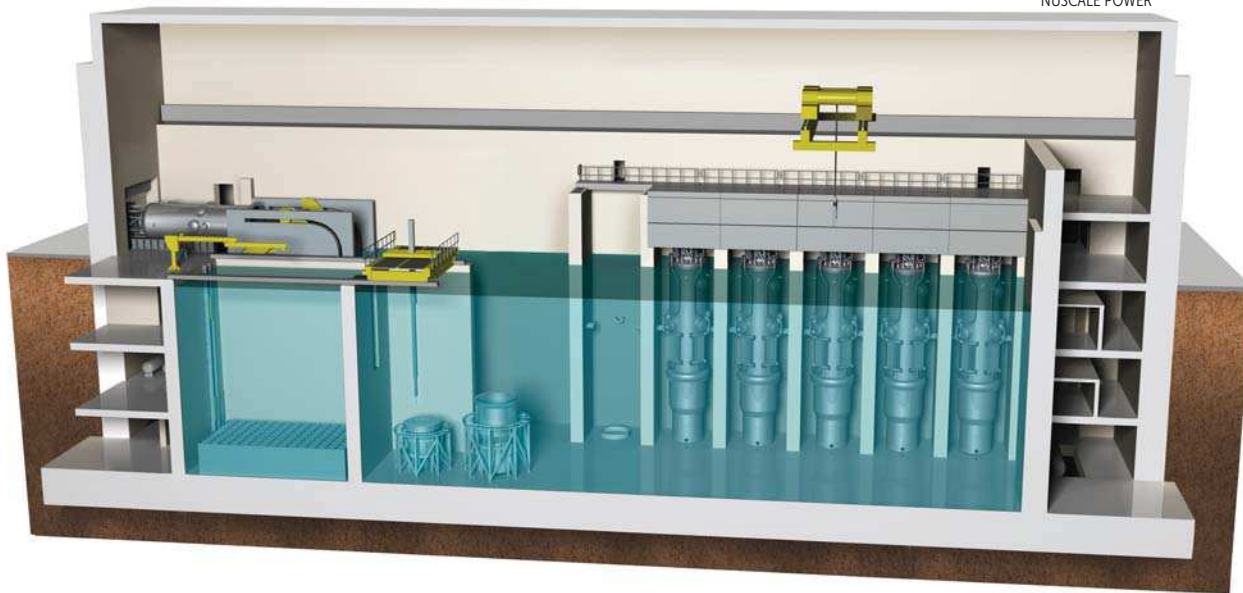
A CROSS-SECTIONAL REPRESENTATION of a NuScale small modular reactor building with five modules installed. A sixth module (left) is in the process of being loaded.
